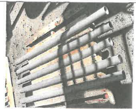
Oil Tubing Excessive wear and pitting
